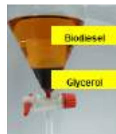
Figure 1: Transesterification of grease trap oil into biodiesel and glycerol (by product).
